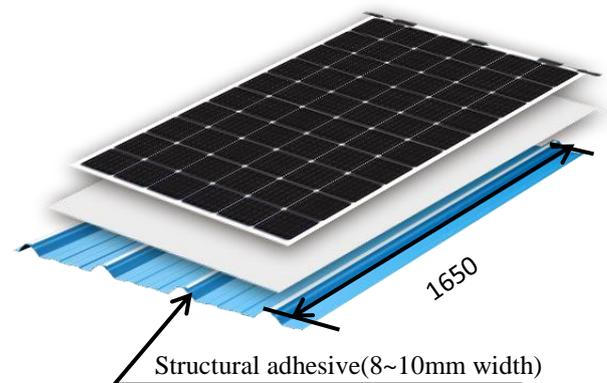
Take tin roof for example, when installing, first inject the industrial structural adhesive to the heave part on 4 tapes of 1650mm long and 8~10mm wide. Laying the flexible modules on the treated surface (see the above picture) and pressing gently against the tile. In order to achieve the best bonding performance, please install the modules within 5 minutes before the adhesive is solidified.
