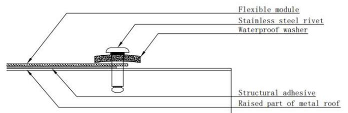
As shown in the figure above, M5 stainless steel rivets are used to successively pass through the waterproof washer, the installation hole in the module and the installation hole in the raised part of the metal roof.Use professional tools to pull out the core of rivets and complete the fixing work.Finally, fill the right amount of waterproof glue at the rivet core area.
